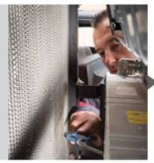
The well proportioned cooling package is easy to access, clean and maintain. 90% of dust is removed naturally thanks to the suction from the cooling fan. The engine air filter is also very easy to access and clean.
