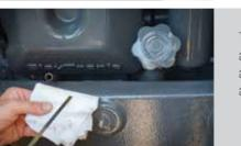
The waisted bonnet and front axle design ensures comfortable access to the engine oil filters and oil dipstick.
