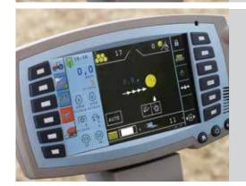
ISOBUS for total implement control – ISOBUS allows an implement manufacturer's control system to be displayed on the console screen, saving owners and operators time and money, with no need to install additional terminals in the cab. Simply plug the implement lead into the tractor's ISOBUS socket and the system automatically uploads the operating menus and displays on the screen – implement control switch assignment on Multipad available (Exclusive version only).
