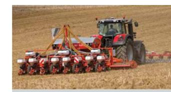
The latest tyre equipment allows MF 8700 models to work at very low tyre pressures, even for high traction jobs, including dual wheels:
