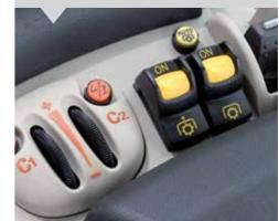
Fender mounted PTO, hydraulic spool valve and linkage controls.
