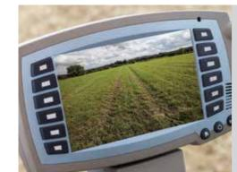
**Video Mode –** Pictures from an on-board camera can be displayed on the console screen, allowing operators to monitor complex implements or simply improve safety and efficiency when reversing.
